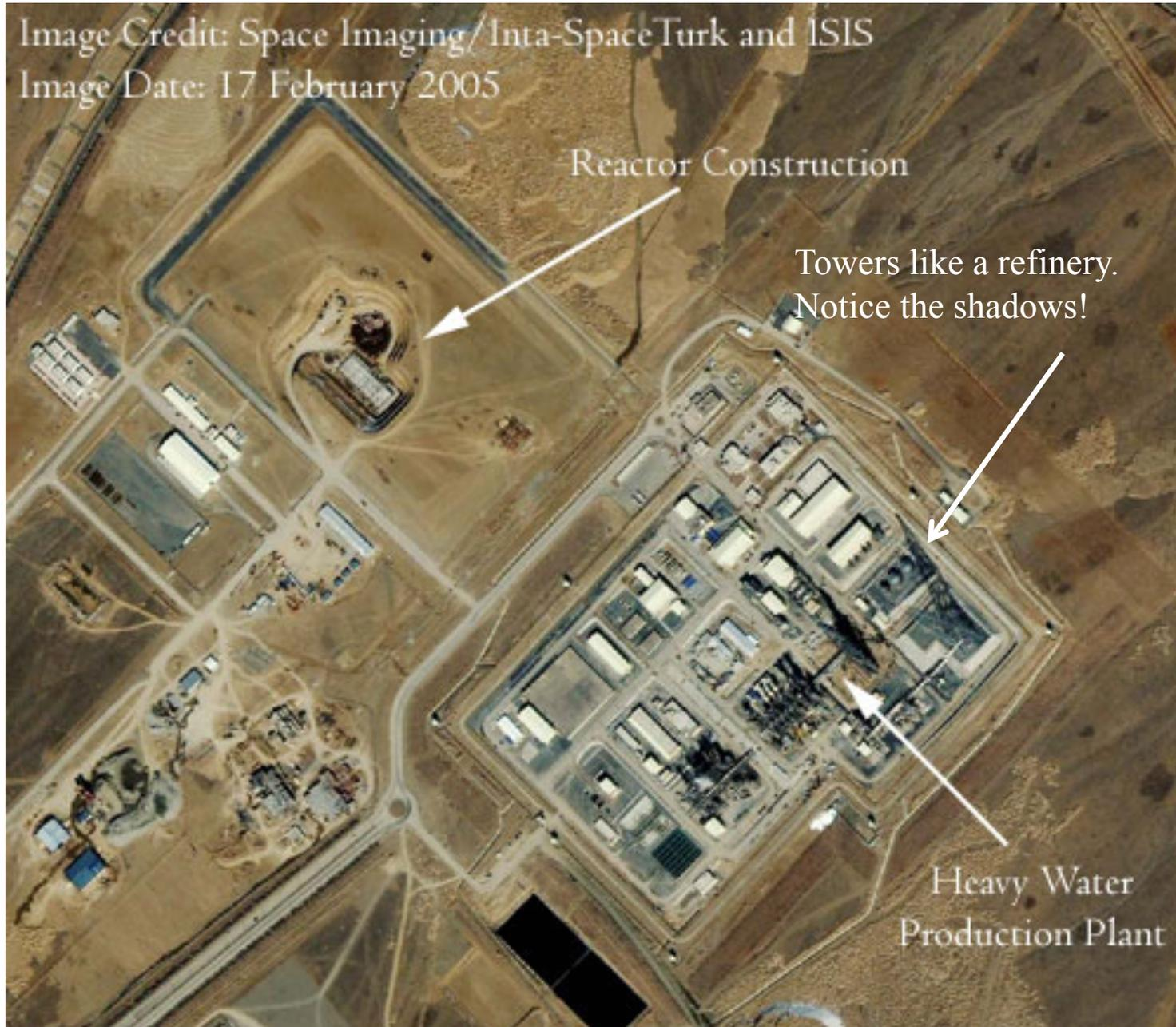
**D<sub>2</sub>O doesn't absorb as many neutrons as H<sub>2</sub>O, so you can make a reactor with natural un-enriched uranium (0.7% U-235) fuel in a tank of heavy water.**
